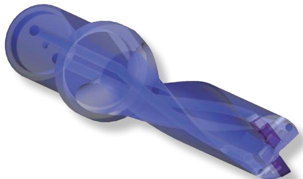
Twisted coolant hole in the drill body increases coolant flow by 1.5 times, which improves chip evacuation, resulting in excellent surface finish.
